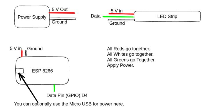
In the crude drawing above, you'll notice that I have setup red as the 5 V out / in, white as the ground, and green as the data wire. Given these things as they are, you simply connect all red together, all white together, and the green together, then plug in the power supply. This should turn on your ESP home and your LED Strip, and allow you to start sending signals to your LEDs.
