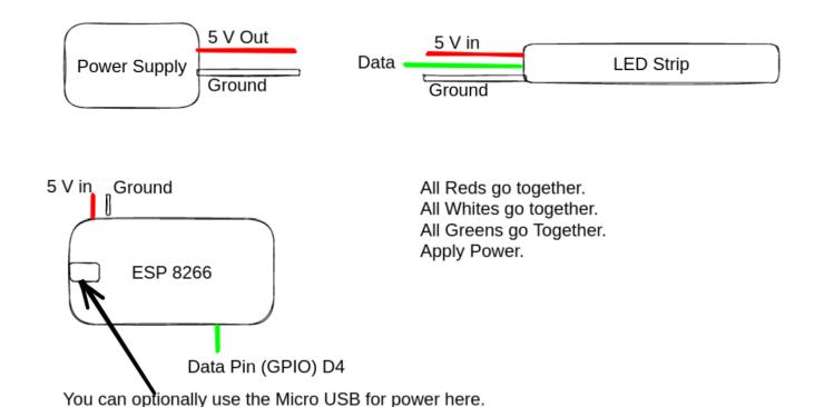
In the crude drawing above, you'll notice that I have setup red as the 5 V out / in, white as the ground, and green as the data wire. Given these things as they are, you simply connect all red together, all white together, and the green together, then plug in the power supply. This should turn on your ESP home and your LED Strip, and allow you to start sending signals to your LEDs.
